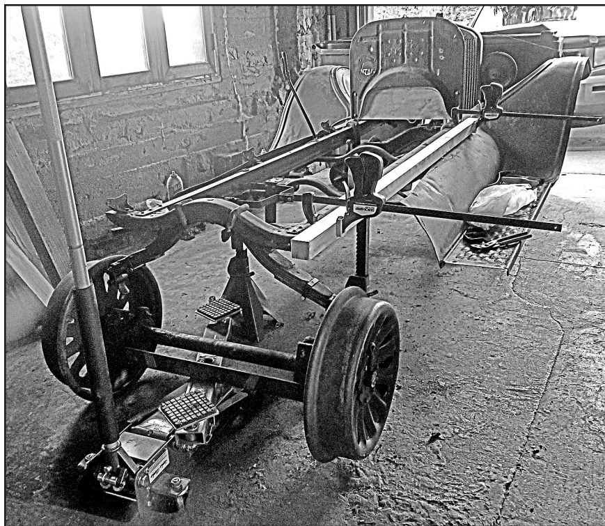
A new wood stringer fitted on the Model T replica. – Photo © 2019 Jeff Badger.
